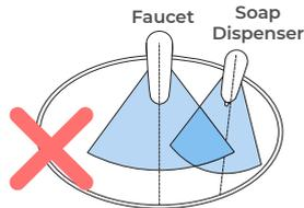
Installing electronic soap dispenser & faucet with intersecting centerline might lead to accidental activation of either or both.
