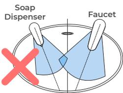
Keep sensor range adjustment within 4 inches away from center of spout. This can only be done with optional remote control.
