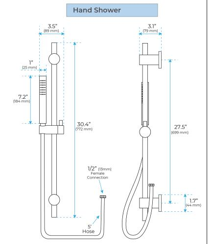
Flow Rate: 2.0 GPM / 7.6 LPM
