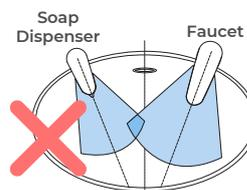
Keep sensor range adjustment within 4 inches away from center of spout. This can only be done with optional remote control.
