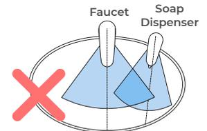
Installing electronic soap dispenser & faucet with intersecting centerline might lead to accidental activation of either or both.
