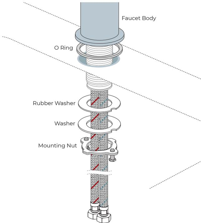
1. Remove the mounting nut, metal washer, and rubber washer from the threaded pipe. Fit the O-ring into the groove of the faucet body. Screw waterlines into the corresponding screw-hole of the faucet body.
