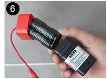
6 Install a universal battery for the battery case and connect the switch device
