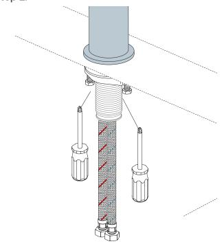
2. Insert waterlines and threaded pipe into the hole of the sink. Install rubber washer, metal washer, and mounting nut back to the threaded pipe. Adjust the faucet body correctly and secure with mounting screws tightly.
