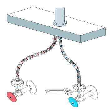
3. Connect waterlines to angle stops. Turn on the angle stops and check for leaks (DO NOT TURN FAUCET ON).
